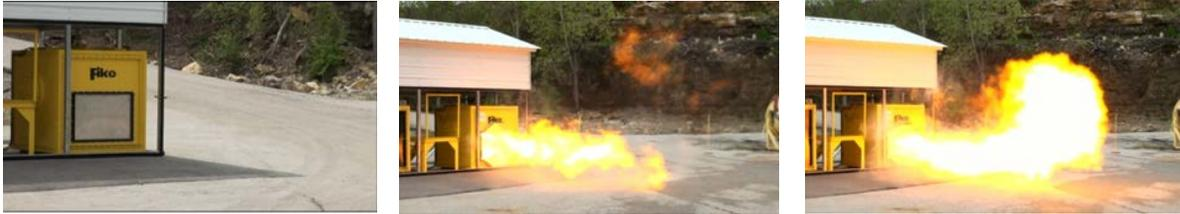
Fig. 2. Dust explosion venting at Fike Remote Testing Facility showing venting with flame release
