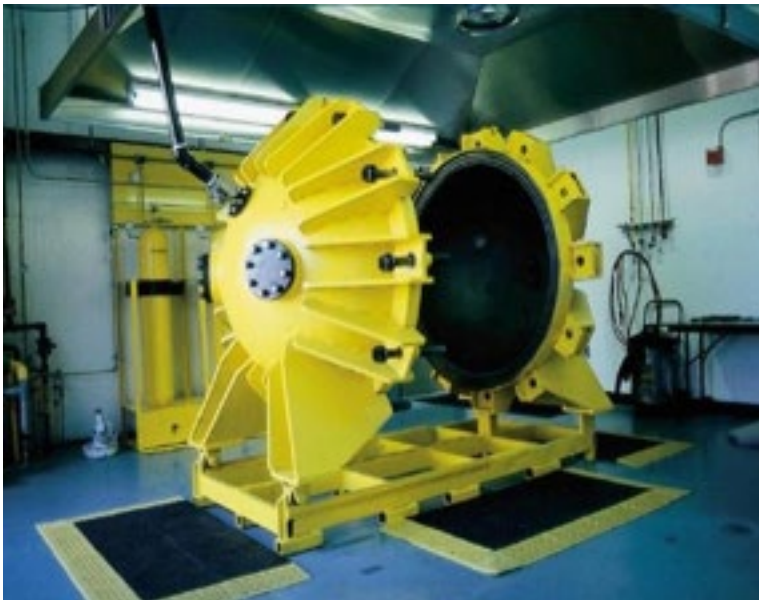
Figure 4: 1-m 3 spherical vessel (Fike Corporation)
