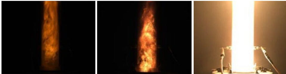
Figure 2: Combustion of cornstarch, iron, and aluminum dusts in a Hartmann tube (Fike Corporation)
